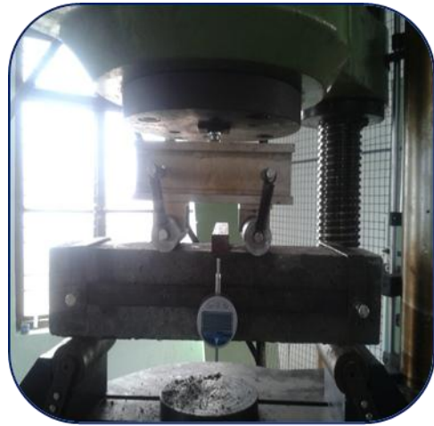
Plate 3. Flexure Test Set-up in UTM
